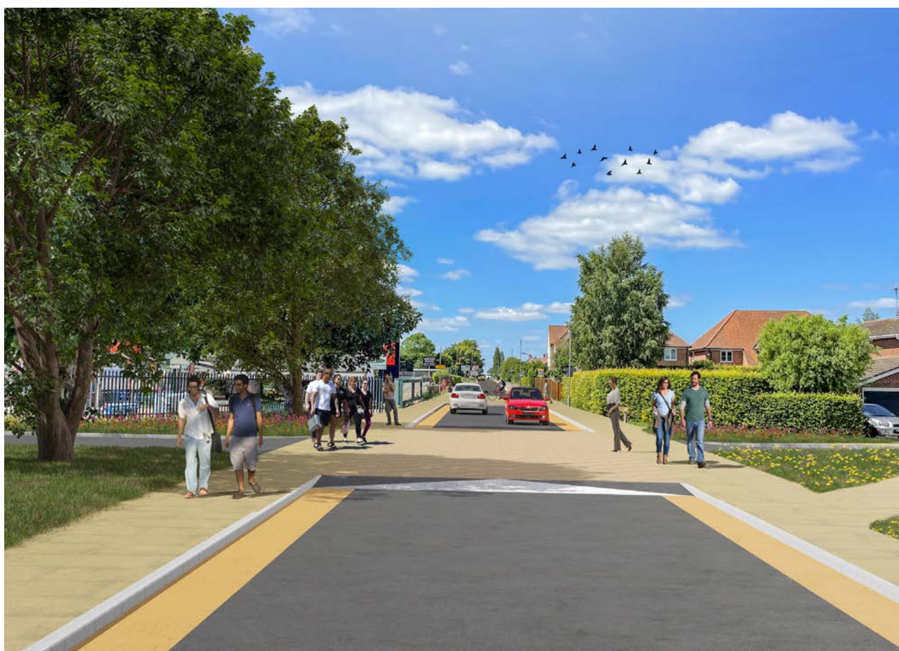
Artists Impression showing a new continuous side road crossing at Wykeham Way
